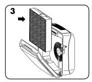
Remove any packaging wrap from the new filters(s) and re-install the filters.
