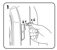
Unlock access panel: to unlock, insert the key provided and rotate counter-clockwise ½ turn.
