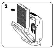
Open front access panel by pressing latches on both sides of unit. Allow panel to open fully. Remove filter(s) to be replaced.
