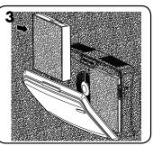
Remove any packaging wrap from the new filters(s) and re-install the filters.
