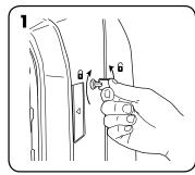
Unlock access panel: to unlock, insert the key provided and rotate counterclockwise ¼ turn.
