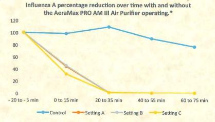
\*Results represent the average of n=3 runs. Device settings A: ionizer ON and filter low speed; device setting B: ionizer off and filter at low speed; device setting C ionizer on and filter at high speed.
